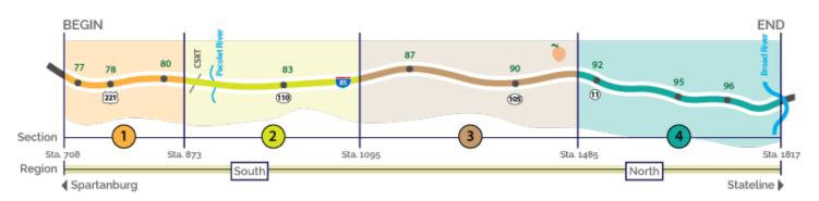
SCDOT, and its two contractors, a Joint Venture of Blythe Construction, Inc. and Zachry Construction Corp. (BZJV) and Lane Construction (Lane), have begun widening and rehabilitation of the existing Interstate 85 beginning at mile marker 77 and continuing to the North Carolina state line.
